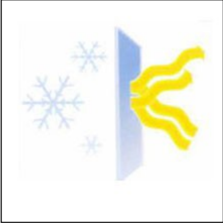
3M All Season Window Films reduce heat loss by reflecting radiant heat back inside the building envelope.
