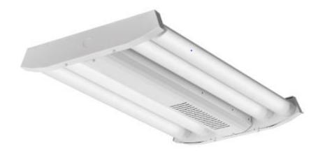
ELECTRICAL — L88 at 60,000 hours L70>100,000 hours. Dtilizes a 90°C case temperature driver for maximum life at high temperatures. 0.90 power factor and 3kA/6kV level of surge protection is standard. Optional 5kA/10kV surge protection available. Available as 120-277V or 347-480V input. 0-10V dimming standard for a dimming range of 100% to 10%.
