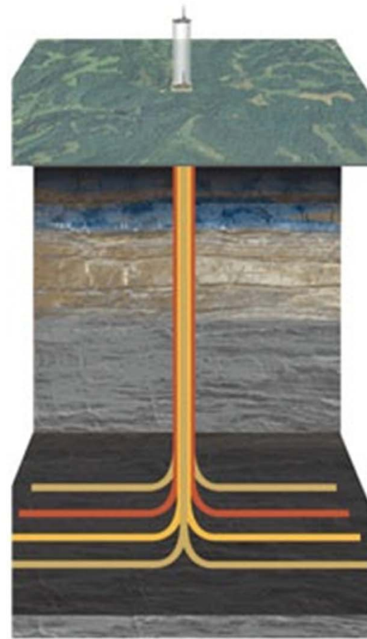
Idealized Horizontal Well Spacing: 1 Padsite Yields Up To 32 Wells.
