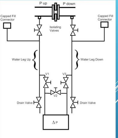
$\Delta P = (Pup + Pwater leg up) - (Pdown + Pwater leg down)$
